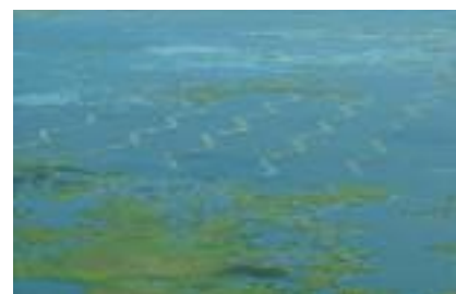
Terraces across Black Lake will protect against erosion and salt water contamination.
